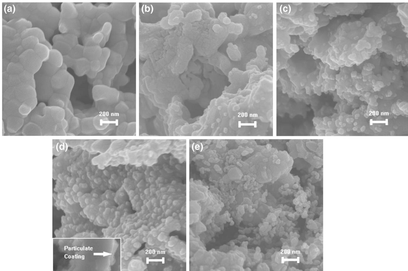
**Fig. 3.** SEM images of the cross-section of LSCF cathodes: (a) blank LSCF; (b) 0.16 mol/L SSC infiltration; (c) 0.48 mol/L SSC infiltration; (d) 1.44 mol/L SSC infiltration; (e) 0.48 mol/L LSCF infiltration.
