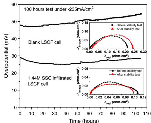
Fig. 6. Comparison of 100 h stabilities between blank LSCF cathode and 4  $\mu\text{L}$  1.44 mol/L SSC-infiltrated LSCF cathode under constant current density of 235 mA/cm<sup>2</sup> at 700 °C.
