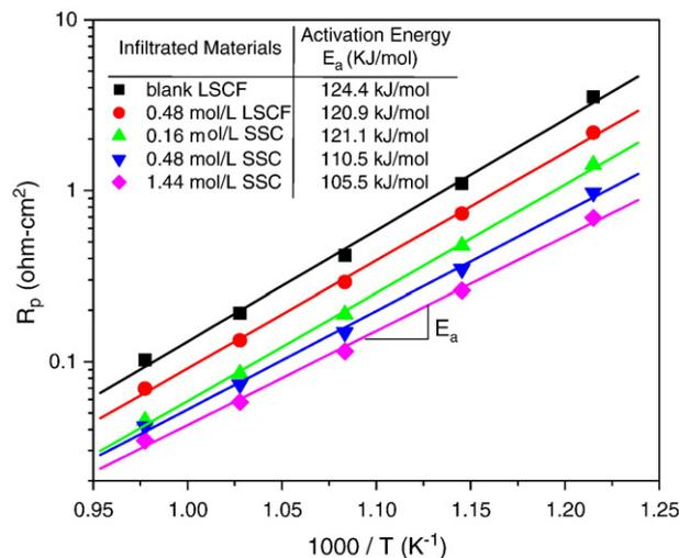
Fig. 5. Interfacial resistances and activation energies as determined from impedance spectra.
