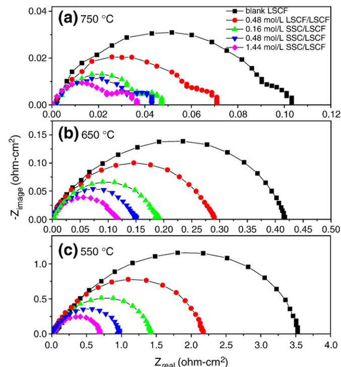
Fig. 4. Impedance spectra of LSCF cathodes with different treatments at various temperatures: (a) 750 °C; (b) 650 °C; (c) 550 °C.
