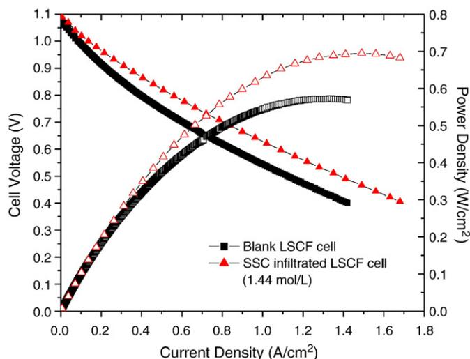
Fig. 7. Cell voltages (solid symbols) and power densities (open symbols) as a function of current densities for blank and SSC-infiltrated LSCF fuel cells operated at 700 °C.
