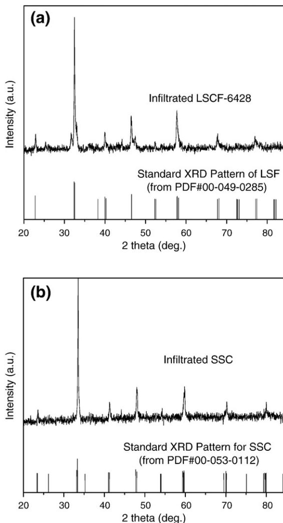
Fig. 1. XRD patterns of infiltrated materials after firing at 850 °C for 2 h: (a) LSCF; (b) SSC.
