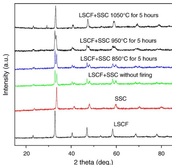
**Fig. 2.** XRD analysis of LSCF and SSC mixture with and without firing at various temperatures for 5 h.
