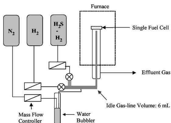
Figure 1. Schematic illustration of the setup for fuel cell testing.
